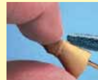
Due to its shape and the coarse cut the D263 KG 60 is well suited for grinding of plaster dies..
