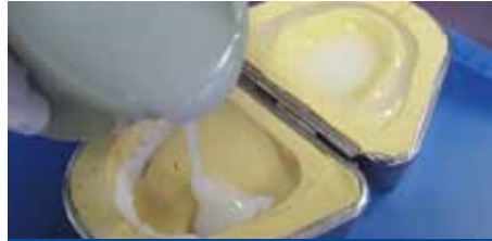
Mix clear acrylic and pour into both sides of mold.
