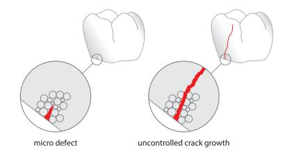
Micro defects on the surface caused by p.e. adjustments after sintering can be the origin of a crack. When the  $K_{IC}$  is exceeded uncontrolled crack growth occurs and lead to fracture. The higher the fracture toughness the higher the resistance against cracks.
