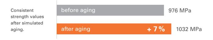
Flexural strength by R&D Dental Direkt GmbH. Test method 3-point bending strength according ISO 6872. Aging according ISO 13356.
